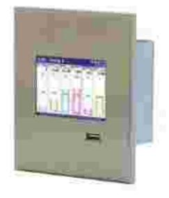
Panel or in-wall mount ITC 8000 CMC-99SL is featured by a shallow casing - only 55 mm! All connectors are introduced on side walls of the device as in a typical panel computer. As the number of measurement inputs and outputs is limited, this design in intended mainly for systems with a small number of signals or systems which include other measurement systems with Modbus RTU interface. An Ethernet interface is also available to upgrade every ITC 8000 control's application easily.
