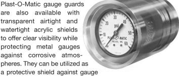
damage caused by external shocks. These shields completely enclose metal gauges and fasteners utilizing an O-ring seal. They can only be used with 2" diameter or smaller gauges and they cannot be used with Plast-O-Matic gauge guards with the removable housing design.
