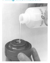
Plast-O-Matic gauge guards purchased with Plast-O-Matic gauges are factory filled. When purchased without a gauge, the installer must ensure that the upper gauge cavity and the gauge or instrument to be used must be solidly filled in order to accurately transmit the process line pressure or vacuum to the instrument. Air
